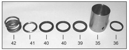
Remove the tension spring (42), support ring (41), v-sleeves (40), pressure ring (39), from the seal sleeve (35). Examine seals (36) carefully and replace if worn. Clean all parts.
