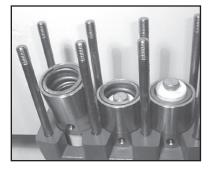
6. Pull seal sleeves (35) out of guides in crankcase (1).
