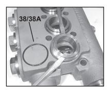
8. Remove seal case (37) from valve casing (43) and inspect O-rings (38/38A).
