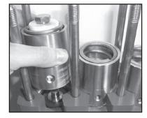
10. Place new plunger pipe (29B) carefully through the oiled seals and push seal sleeve (35) with plunger pipe into the crankcase guide. *Note: Make sure weep hole is facing down.*
