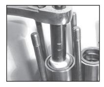
Tighten the tension screws (29C) to 310 in.lbs. (35NM). The plunger pipe (29B) should not be strained by over tightening of the tension screw (29C) or through damage to the front surface of the plunger; otherwise, it will probably break.
