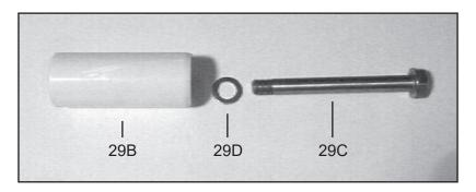
9. Check plunger surface (29B). If plunger pipe is worn, loosen tension screws (29C) and pull off plunger pipe to the front. Clean front surface of plunger (25) thoroughly. Apply a thin coat of Loctite to the tension screw threads (29C). Note: Care must be taken that no glue gets between the plunger pipe (29B) and the centering sleeve (29A). Add new copper ring (29D).
