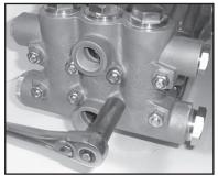
Loosen the 8 nuts (49A) with a 19mm wrench. Tap the back of the manifold (43) with a rubber mallet to dislodge and slide off the studs (49).
