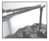
12. Place valve vasing (43) over studs and push firmly until seated against the crankcase (1). Tighten the hexagon nuts (49A) in a crosswise pattern (shown below) to 59 ft.-lbs. (80 NM)
