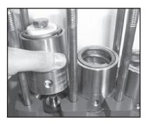
Place new plunger pipe (29B) carefully through the oiled seals and push seal sleeve (35) with plunger pipe into the crankcase guide. Reconnect rinsing system.
