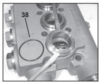
8. Remove seal case (37) from valve casing (43) and inspect O-rings (38).
