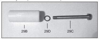
worn, loosen tension screws (29C) and pull off plunger pipe to the front. Clean front surface of plunger (25) thoroughly. Apply a thin coat of Loctite to the tension screw threads (29C). **Note:** Care must be taken that no glue gets between the plunger pipe (29B) and the centering sleeve (29A). Add new copper ring (29D).
