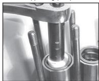
Tighten the tension screws (29C) to 310 in.-lbs. (35NM).
