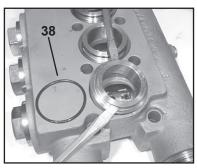
8. Remove seal case (37) from valve casing (43) and inspect O-rings (38).
