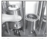
Place new plunger pipe (29B) carefully through the oiled seals and push seal sleeve (35) with plunger pipe into the crankcase guide. Note: Make sure weep hole is facing down.
