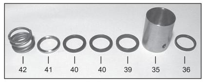
7. Remove the tension spring (42), support ring (41), v-sleeves (40), pressure ring (39), from the seal sleeve (35). Examine seals (36) carefully and replace if worn. Clean all parts.
