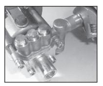
With a crescent wrench, remove the injector retainer (47). Inspect the o-ring (46) for wear and replace as necessary.
