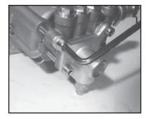
4. Next, remove the four manifold bolts (40) with a 6mm allen wrench.
