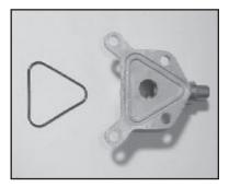
Remove the suction flange 6. (39) and flange o-ring (38). Inspect the o-ring for wear and replace as necessary.
