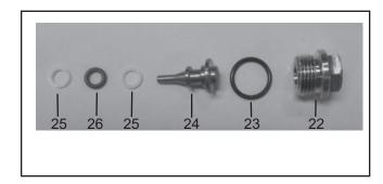
7. Remove the piston (24), o-ring (26), and backup rings (25). Remove the bypass valve seat (28). Inspect the parts for wear and replace as necessary. **IMPORTANT! Make sure that the shoulder on bypass valve seat (28) is facing the discharge plug (22).**
