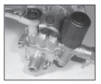
With a 14mm socket wrench, remove the three discharge valve plugs (22). Inspect the valve plug o-rings (23) for wear, and replace as necessary.
