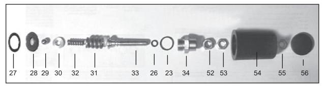
4. With a 19mm wrench, remove the adjusting screw plug (34). Unscrew the adjusting screw (33) from the adjusting screw plug (34). Inspect the o-rings (23 & 26) for wear and replace as necessary.
