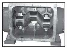
13) Push connecting rod halves together with the crosshead as far as possible into the crosshead guide. Take out bearing cover (14/14A) and push out crank-shaft taking particular care that the con rod doesn't get bent. Check surfaces on the connecting rods (24), crankshaft (22) and crossheads (25). Check the surfaces of the crosshead guides in the crankcase for any unevenness.
