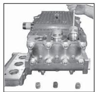
Take out pressure springs (57A). Pull out assembled valves (51 & 52) with valve pulling tool (07662).
