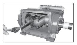
12) Remove the connecting rod screws (24). Important! Connecting rods are marked 1 to 3 for identification. Do not twist connecting rod halves or interchange them. When reassembling, the connecting rod must be fitted in their exact original position on the crankshaft journals.
