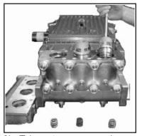
Take out pressure springs (57A). Pull out assembled valves (51 & 52) with fitting tool.
