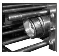
8) Take out the seal case (38) from the valve casing (if necessary secure 2 screwdrivers in the front O-ring groove to extract seal case). Coat seals with silicon grease before installing.
