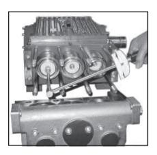
9) Coat the seal sleeve lightly with anti-corrosive grease (e.g. molycote no. Cu-7439) in its fitted area towards the crankcase. Insert the seal sleeves in to their crankcase fittings. Coat the threads of the tension screw (36C) lightly with thread glue and insert it together with a new copper ring (36D) through the ceramic pipe. Turn the pump per hand until the plunger (25) rests against the plunger pipe. Tighten the tension screw at 30 Ft-lbs. (40 Nm).
