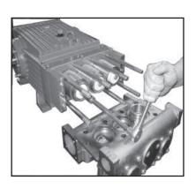
6) Remove tension screw (36C) and take seal sleeve (39) together with all mounted parts out of the drive. Pull plunger pipe out of the seal assembly and check for any damage. Carefully, remove seal rings (40) and sleeves (42) with a screw driver.
