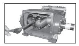
12) Remove the connecting rod screws (24).
