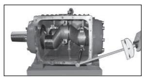
14) Reassemble in reverse order. Thread the long end of the crankshaft together with the inner bearing rings into the crankcase; then mount outer bearing ring (20) and spacer ring (22A). Mount connecting rod halves in their exact original position and tighten at 37 Ft-lbs. (50 Nm). Important! Connecting rods must be able to move slightly sideways on the stroke journals.
