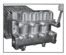
5) Remove hexagon nuts (49A) and valve casing together with seal case (38) from crankcase (1). If necessary, carefully tap the valve casing (50) past the centering stud (50A) using a rubber hammer.
