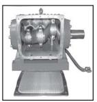
10) Take out plungers and seal sleeves as described above. Drain the oil by taking off the plug (12). After removing the clip ring (33B), lever out the seal retainer (33) with a screwdriver. Open hose adapter (K11) and remove gear cover (K3). Remove the cooling vane plate (K1) by removing the screws (K4)
