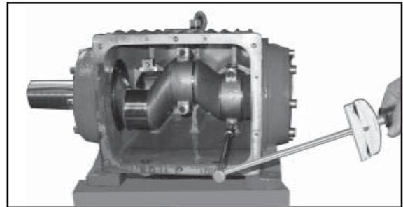
13) Reassemble in reverse order. Thread the long end of the crankshaft together with the inner bearing rings into the crankcase; then mount outer bearing ring (20) and spacer ring (22A). Mount connecting rod halves in their exact original position and tighten at 37 Ft-lbs. **Important!** Connecting rods must be able to move slightly sideways on the stroke journals.
