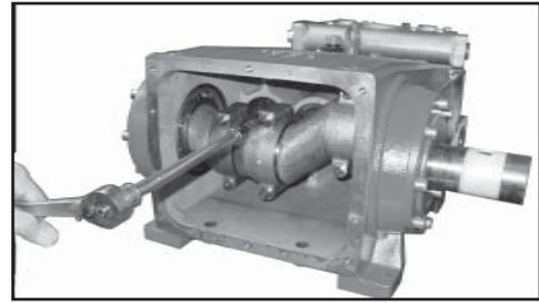
11) Remove the connecting rod screws (24).
