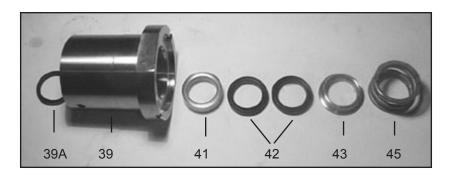
10. Take tension spring (45) and seal pack (41, 42, 43) out of seal sleeve. Take a thin screw driver and pry out the grooved ring (39A). Note: This seal (39A) will not be reusable, so replace with a new part. For the seal-pack (41-43), remove with either a socket wrench or use a screw driver to push against the rear lip of the pressure ring (41) or v-sleeves (42). You will need to remove seals evenly out of the seal sleeve (39). Be careful not to score the sleeve or metal parts (41 & 43).
