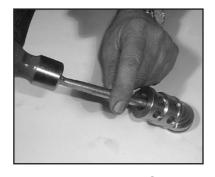
3. Valve seats (51C and 52C) are pressed out of spacer pipe (51F) by hitting the valve plate (51D/52D) with a bolt.
