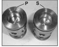
When reassembling: The suction valve seat (51C) is 1mm smaller in diameter than the discharge valve seat (52C). Suction valve seats are marked "S" and always have to be installed first. Discharge valve seats are marked "P" and are always tobe installed on top of suction valve. Plugs (58) are to be tensioned down evenly with screws (58C) in a crosswise pattern at 155 ft-lbs. (210 Nm).
