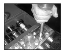
2. Take out tension spring (57) and complete valve (51) using either valve tool (part #07662) or stud bolt M16.
