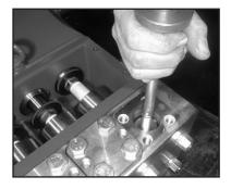
Take out tension spring (57) and complete valve (51) using either valve tool (part #07662) or stud bolt M16.
