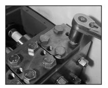
Loosen screws (58C), take plugs (58) out of valve casing with two screws.
