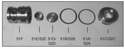
Check surfaces of valve plate (51D/52D), valve seat (51C/52C), O-rings (51B, 58A), and support rings (51A, 58B) and replace worn parts.
