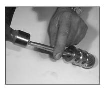
Valve seats (51C and 52C) are pressed out of spacer pipe (51F) by hitting the valve plate (51D/52D) with a bolt.
