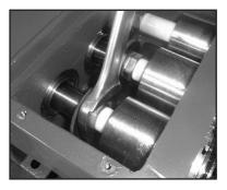
Separate plunger (36A) from crosshead (25) by means of one open-end wrench (M36).
