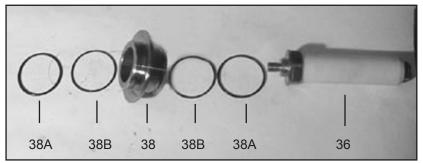
11. Check plunger pipe (36B) and seals (39A, 42) for wear. When replacing plunger pipe (36B), tighten tensioning screw (36C) to 30 ft-lbs (40 NM). If o-rings (38A) or support rings (38B) are damaged, replace with new parts.
