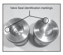
7) When reassembling: The inlet valve seat (51C) is 1mm smaller in diameter than the discharge valve seat (52C). Inlet valve seats are marked "S" and always have to be installed first. Discharge valve seats are marked "P" and are always to be installed on top of inlet valve. Plugs (58) are to be tensioned down evenly with screws (58C) in a crosswise pattern at 155 ft.-lbs. (210 Nm).
