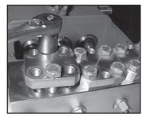
2) Take plugs (58) out of valve casing (50) by tightening screws (58C) against valve casing with two screws.
