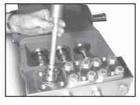
4) Take out valve assemblies (51 & 52) using either valve tool (part #07662) or a stud bolt (M16).
