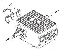
Important! Do not bend connecting rod shafts. Check the running surface of the shaft and connecting rods as well as the shaft seal rings and tapered roller bearings.
