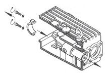
Important! Connecting rods are marked for identification. Do not twist connecting rod halves. When reassembling, connecting rods are to be fitted back onto the shaft journals in their exact original position.
