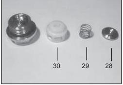
Remove the exposed spring tension cap (30) from valve seat by pushing it sideways with a screwdriver. Remove spring tension cap (30), valve spring (29), and valve plate (28).
