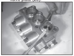
Using two screwdrivers, remove seal case (21)
