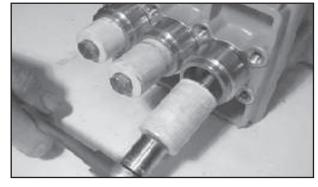
10. If the plunger pipe (16B) is worn, remove tension screw (16D) and remove together with plunger pipe. Check and clean plunger (16A) surfaces and mount new plunger pipe. Cover thread of tension screw (16D) with a thin film of Loctite and tighten carefully at 247 in-lbs (28 Nm).
