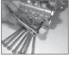
4. Remove hexagon socket screws (34) and remove valve casing (26) by pulling them frontwise over the plungers (16)
