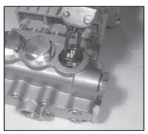
Pull out valve seat (27) and O-ring (31) with a valve puller. Check O-ring for wear.
