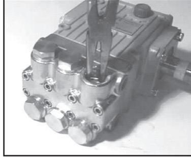
2. Using a needle nose pliers, remove the inlet and discharge valve assemblies (27-30). Inspect all parts for wear and replace as necessary.
