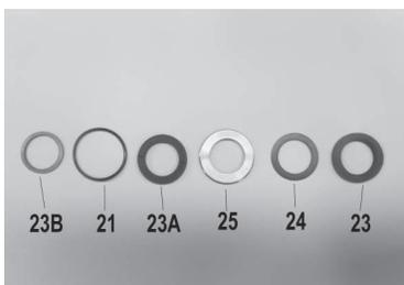
7. Remove the weep return ring (25), pressure ring (24), and v-sleeve (23) from the valve casing (26). Remove the rear v-sleeve (23A) and drip shield (23B) from the seal case (20). Inspect all parts, including o-ring (21) for wear and replace as necessary.
