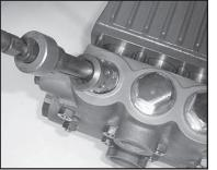
2. Remove the complete valve assembly (46) with valve pullers.
