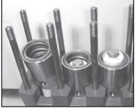
5. Pull seal sleeves (35) out of guides in crankcase (1).
