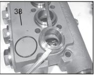
7. Remove seal case (37) from valve casing (43) and inspect o-ring (38).
