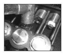
6. Remove pump head by tapping from the back with a rubber mallet.
