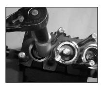
10. Remove tension screw (29C) and remove the plunger pipe from centering sleeve (29A)
