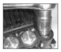
1. Remove plugs (48) with a 36mm wrench and check o-ring (44A) and support ring (44B) take out spring (45).
