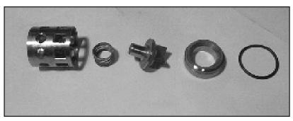
4. Unscrew the valve seat, remove the valve plate (46B) and spring (46C). The seal ring (46E) is snapped onto the valve plate. Check all sealing surfaces and replace worn parts. Tighten plugs (48) to 107 ft-lbs. (145 Nm).
