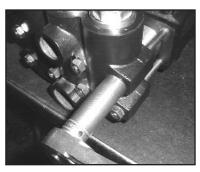
13. Tighten hexagon nuts (49A) in a crossing pattern shown to the right to 59 ft.-lbs. (80 Nm).
