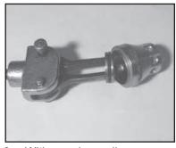
With a valve puller remove the valve seat (37) and oring (38). If excessive pitting is seen, replace the worn parts. Check valve seat o-ring (38) for wear and replace as necessary.
