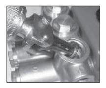
3. Use a small slide hammer to remove valve seats (37) from manifold (29). Inspect valve plate (36) and valve seats (37) for wear. If excessive pitting is seen, replace the worn parts. Check valve seat o-ring (38) for wear and replace as necessary.
