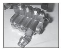
6. Remove the inlet valve retainer assembly (34A-39)
