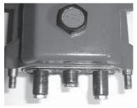
13.Before replacing pump manifold (29), first rotate crankshaft (18) until two outside plungers (24A) extend evenly forward. Lubricate ceramic plungers with a light film of oil. Carefully and evenly slide manifold over plungers and press manifold firmly against crankcase (1). Replace manifold stud bolts (45), washers (47) and nut (46) and tighten to 59 ft.-lbs. (80 Nm).
