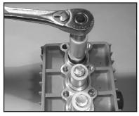
10) If the plunger pipe (16B), is damaged or worn, remove tension screw (16D) and plunger pipe (16B). Check and clean plunger surface (16A) and check flinger (16H). Cover thread of tension screw (16D) with a thin film of Loctite and tighten carefully to 20.7 ft.-lbs. (28 Nm).
