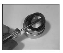
8) Remove the weep grooved seal (23) out of the seal case (20). Check O-rings (21).
