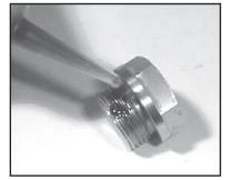
Remove the o-ring (31). Inspect all parts for wear and replace as necessary. Apply one drop of loctite 243 to the valve plugs (32) and tighten to 107 ft.-lbs. (145 NM).
