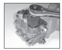
With a socket wrench, remove the three discharge valve plugs and three inlet valve plugs (32). Inspect the o-ring (33) for wear and replace if damaged.
