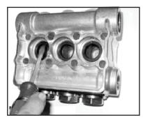
Remove the pressure rings (24) and v-sleeves (23 - Note: P422 & P423 pumps have a spacer ring) from the valve casing (26).
