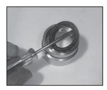
Remove the weep grooved seal (23) out of the seal case (20). Check O-rings (21).
