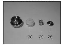
Remove the exposed spring tension cap (30) from valve seat by pushing it sideways with a screwdriver. Remove spring tension cap (30), valve spring (29), and valve plate (28).
