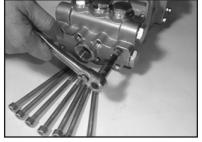
Remove hexagon socket screws (34) and remove valve casing (26) by pulling them frontwise over the plungers (16).
