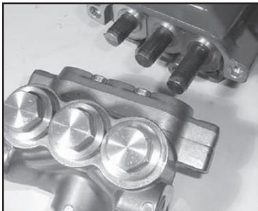
6. With a rubber mallet tap the back of the valve casing (29) and pull the valve casing (29) off the plungers (24A).
