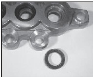
17. Lubricate the weep seal (50) and install into the intermediate casing (48).
