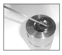
10) Remove leakage seal (36) from the seal sleeve. If worn or damaged replace with new seal.
