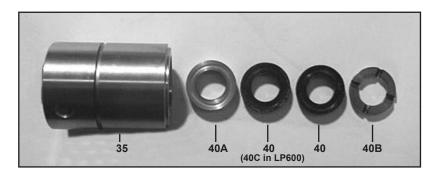
11) Remove the pressure ring (40A), v-sleeves (40), sleeve, and support ring (40B), from the seal sleeve. For LP301A and LP301A-4000 pumps, remove the pressure spring (41). Examine seals carefully and replace if worn. Clean surfaces of seal sleeves (35) which come in contact with the crankcase (1) and sealing surfaces of valve casing (43).
