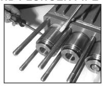
7) Remove the seal sleeve (35) from the manifold and /or crankcase.
