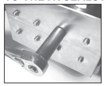
6) Loosen the 8 nuts (49A) with a 19mm socket and pull off valve casing (43) to the front.
