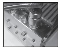
5) Tighten up tension plugs (48) to 107 ft.-lbs. (145 NM)
