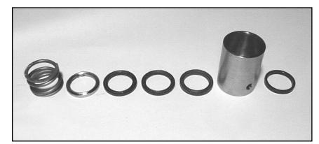
Remove the tension spring (42), support ring (41), v-sleeves (40), pressure ring (39), from the seal sleeve (35). Examine seals (36) carefully and replace if worn. Clean all parts.
