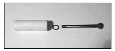
10) Check plunger surface (29B). If plunger pipe is worn, loosen tension screws (29C) and pull off plunger pipe to the front. Clean front surface of plunger (25) thoroughly. Apply a thin coat of Loctite to the tension screw threads (29C). **Note: Care must be taken that no glue gets between the plunger pipe (29B) and the centering sleeve (29A).** Add new copper ring (29D).
