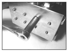
6) Loosen the 8 nuts (49A) with a 19mm socket and pull off valve casing (43) to the front.
