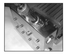
Take out discharge valve assemblies (46) by pulling them upwards out of the valve casing (43) with a snap-ring tongs or any other pull-off device. Then remove inlet valves in the same way.
