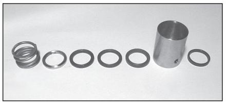
8) Remove the tension spring (42), support ring (41), v-sleeves (40), pressure ring (39), from the seal sleeve (35). Examine seals (36) carefully and replace if worn. Clean all parts.
