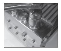
5) Tighten up tension plugs (48) to 107 ft.-lbs. (125 NM)
