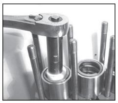
12) Tighten the tension screws (29C) to 310 in.-lbs. (35NM). The plunger pipe (29B) should not be strained by over tightening of the tension screw (29C) or through damage to the front surface of the plunger; otherwise, it will probably break.
