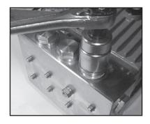
Loosen and remove tension plugs (48) with a 36mm socket wrench.
