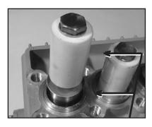
9) Check surfaces of plunger (16). Damaged surfaces cause accelerated seal wear. Deposits of all kinds must be removed from the plungers.
