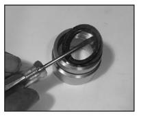
8) Remove the weep grooved seal (23B) together with pressure ring out of the seal case (20). Check O-rings (21).
