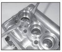
6) Remove seal adapters (20) and weep return rings (25) from the valve casing.
