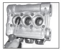
7) Remove the pressure rings (24) and v-sleeves (23).
