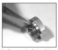
4) Remove the O-ring (31). Inspect all parts for wear and replace as necessary. Apply one drop of loctite 243 to the valve plugs (32) and tighten to 107 ft.-lbs. (145 NM).
