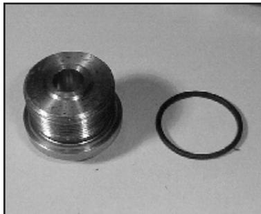
2. Inspect the plug o-rings (#48A and #42B) and replace as necessary.
