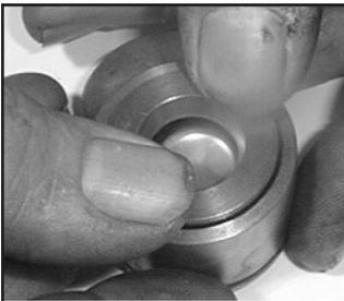
18. Reassemble the discharge valve assembly by placing the valve plate (#45), spring (#46), and spring retainer (#47) on top of the valve seat (#44). Press fit together. Place the entire discharge assembly into discharge port making certain the assembly is properly seated. Replace discharge plug (#48) and tighten securely.
