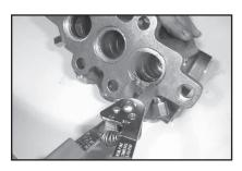
15. Replace the rear v-sleeve assembly (#35A-35D) and replace the snap ring (#36).
