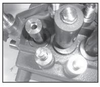
12. Inspect the crankcase oil seals (#31) for evidence of leaking. If there is oil on the crankcase (#1) at the sight of the oil seals, they must be replaced. The oil seals are replaced after removing the crosshead/plunger assembly (#25) as described on page 9.
