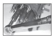
14. Torque the ceramic plunger bolt assembly to 300 inch-pounds (34 Nm). If originally removed, reinstall the stud bolts (#49).
