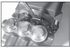
5. Remove the six manifold stud nuts (#50) with a 19mm wrench. Remove the spring washers (#50A). Tap the back of the manifold with a rubber mallet to dislodge and slide it off the studs (#49). The spacer (#51) can now be removed by prying gently outward with a screwdriver through the front of the inlet port.
