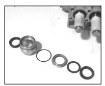
Remove the weep return ring (25), pressure ring (24), and v-sleeve (23) from the valve casing (26). Remove the rear v-sleeve (23A) from the seal case (20). Inspect all parts, including o-ring (21) for wear and replace as necessary.
