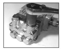
With a 22mm socket wrench, remove the (3) discharge valve plugs and (3) inlet valve plugs (32) Inspect the o-ring (33) for wear and replace if damaged.
