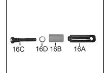
Check surfaces of plunger pipe (16B). A damaged surface will cause accelerated wear on the seals. Deposits of any kind must be carefully removed from the plunger surface. A damaged plunger must be replaced!
