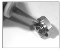
Apply one drop of Loctite 243 to the valve plugs (32) and tighten to 55 ft.-lbs. (75 Nm).
