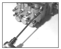
Next, use a 5mm allen wrench to remove the 8 socket head cap screws (34).
