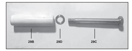
12) Check plunger surface (29B). If plunger pipe is worn out, loosen tension screws (29C) with a 15mm socket and pull off plunger pipe to the front. Clean front surface of plunger (29B) thoroughly. Apply a small drop of locktite to tension screw. Put a **new** crush washer (29D) onto tension screw. Put a thin coat of glue (Loctite) on the ring (or ceramic plunger side) and tighten screw to 265 in.-lbs. (30 NM).
