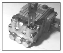
Using a needle nose pliers, remove the inlet and discharge valve assemblies (26A) and o-ring (31). Inspect all parts for wear and replace as necessary.
