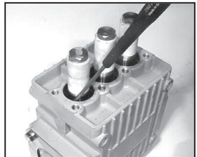
9. If the crankcase oil seals (19) are to be replaced, they can be removed by prying loose with a flat screwdriver. Take care not to make contact with the plunger.
