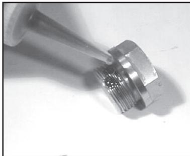
4. Apply one drop of Loctite 243 to the valve plugs (32) and tighten to 55 ft.-lbs. (75 Nm).
