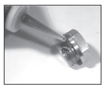
4. Apply one drop of Loctite 243 to the valve plugs (32) and tighten to 55 ft.-lbs. (75 Nm).
