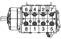
Important! The torque tension on the screws (49A) must be checked after 8-10 operating hours; the pump must be at zero pressure. Thereafter, the tension is to be checked every 200 operating hours.
