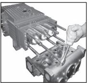
6) Remove tension screw (36C) and take seal sleeve (39) together with all mounted parts out of the drive. Pull plunger pipe (36B) out of the seal assembly and check for any damage. Carefully, remove seal rings (40) and sleeves (42) with a screwdriver.
