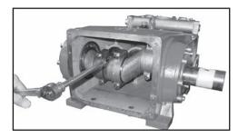
12) Remove the connecting rod screws (24). Important! Connecting rods are marked 1 to 3 for identification. Do not rotate connecting rod halves or interchange them. When re-assembling, the connecting rod must be fitted in their exact original position on the crankshaft journals.
