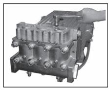
1) Remove socket head cap screws (58)
