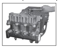
1) Remove socket head cap screws (58)
