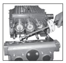
9) Coat the seal sleeve(39) lightly with anti-corrosive grease (e.g. molycote no.Cu-7439) in its fitted area towards the crankcase. Insert the seal sleeves in to their crankcase fittings. Coat the threads of the tension screw (36C) lightly with thread glue and insert it together with a new copper ring (36D) through the ceramic pipe. Turn the pump by hand until the plunger (25) rests against the plunger pipe. Tighten the tension screw at 30 Ft-lbs. (40 NM)
