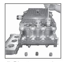
3) Take out pressure springs (57A). Pull out assembled valves (51 & 52) with valve puller.
