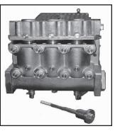
2) Lift discharge casing (50B) up and away.
