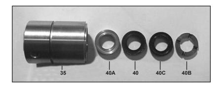
11) Remove the pressure ring (40A), v-sleeves (40/40C), sleeve, and support ring (40B), from the seal sleeve. Remove the pressure spring (41). Examine seals carefully and replace if worn. Clean surfaces of seal sleeves (35) which come in contact with the crankcase (1) and sealing surfaces of valve casing (43).
