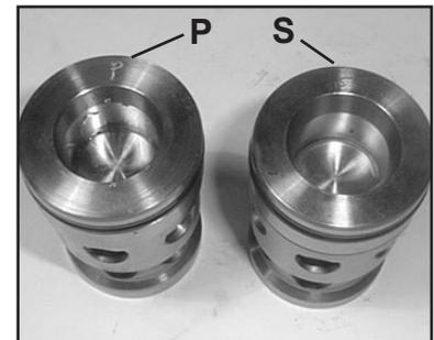
5. When reassembling: The suction valve seat (51C) is 1mm smaller in diameter than the discharge valve seat (52C). Suction valve seats are marked "S" and always have to be installed first. Discharge valve seats are marked "P" and are always to be installed on top of suction valve. Plugs (58) are to be tensioned down evenly with screws (58C) in a crosswise pattern at 155 ft-lbs. (210 Nm).
