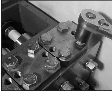
1. Loosen screws (58C), take plugs (58) out of valve casing with two screws.
