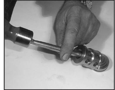
3. Valve seats (51C and 52C) are pressed out of spacer pipe (51F) by hitting the valve plate (51D/52D) with a bolt.
