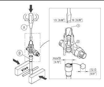
ton housing (13) insert a 13mm socket (max. 3/4" ID) into by-pass port and onto hexagonal part of piston. Secure in place. Using a flat blade screwdriver (10mm wide x 1.5mm), insert fully into slot on top of piston housing (tap into place with a hammer, if needed, to seat completely). Turn to unthread until parts are separated.
