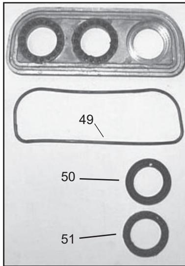
11. Inspect seals (50), seal support ring (51) and O-ring (49) and replace as necessary.
