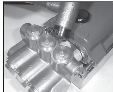
5. Tap the back of the valve casing (29) with a rubber mallet.
