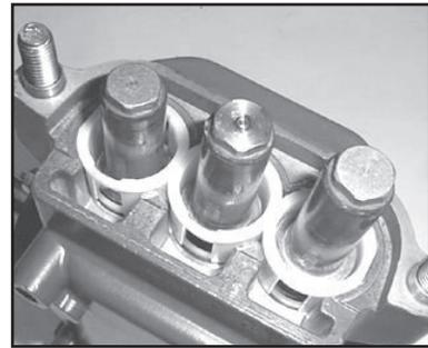
12. Inspect ceramic plunger (24A) tips for wear. If necessary, replacement of the ceramic plungers may be accomplished by removing the plunger bolt assemblies (24) with a 13mm wrench. Ceramic plungers should now slide off the stainless steel plunger base (22). Excessive resistance to plunger removal may be overcome by heating the stainless steel plunger base. This will melt any excess loc-tite beneath the ceramic plunger allowing easy removal.
