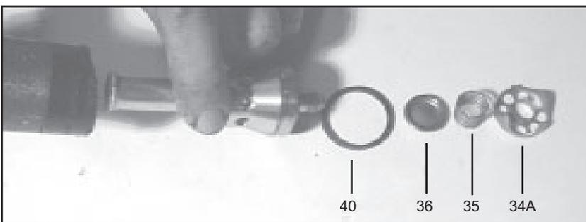
7. Remove the o-ring, (40), valve plate (36), valve spring (35), spring retainer (34A). Check valve retainer o-ring (40) for wear.
