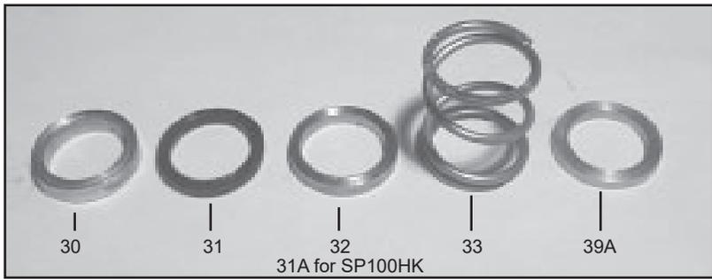
9. Remove the spacer (39A), pressure spring (33), support ring (32 or 31A for SP100HK), v-sleeve (31), and pressure ring (30), from the manifold (29) and check for wear.
