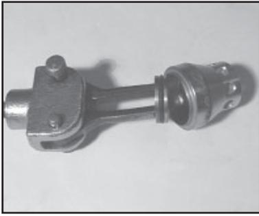
8. With a valve puller remove the valve seat (37) and o-ring (38) replace if worn. If excessive pitting is seen, replace the worn parts. Check valve seat o-ring (38) for wear and replace as necessary.
