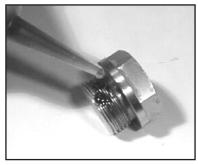
4) Remove the o-ring (31). Inspect all parts for wear and replace as necessary. Apply one drop of Loctite 243 to the valve plugs (32) and tighten to 107 ft.-lbs. (145 Nm) for P420-3100/ P423-3100 and 125 ft-lbs (170 Nm) for P435-3100/ P450-3100).
