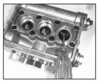
7) Remove the pressure rings (24) and v-sleeves (23 - Note: P423-3100 pumps have a support ring) from the valve casing (26).
