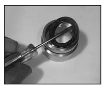
8) Remove the weep grooved seal (23 or 23B) together with pressure ring (24 - P420 -3100 only) out of the seal case (20). Check O-rings (21).
