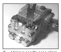
Using a needle nose pliers, remove the inlet and discharge valve assemblies (27-30), for P230-3100 only, remove spacer (30A), and o-ring (31). Inspect all parts for wear and replace as necessary.
