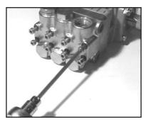
Next, use a 5mm allen wrench to remove the 8 socket head cap screws (34).
