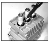
If the crankcase oil seals (19) are to be replaced, they can be removed by prying loose with a flat screwdriver. Take care not to make contact with the plunger.
