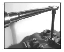
12. Place valve vasing (43) over studs and push firmly until seated against the crankcase (1). Tighten the hexagon nuts (49A) in a crosswise pattern (shown below) to 59 ft.-lbs. (80 NM)
