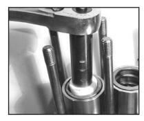
11. Tighten the tension screws (29C) to 310 in.lbs. (35NM). The plunger pipe (29B) should not be strained by over tightening of the tension screw (29C) or through damage to the front surface of the plunger; otherwise, it will probably break.
