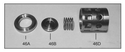
4. Loosen valve seats (46A) from spacer pipe (46D) by lightly hitting the valve plate (46B) with a plastic stick. Check sealing surface and replace worn parts. Reassemble with new O-rings (44A) and oil them before installing. Tighten up tension plugs (48) to 107 ft.-lbs. (145 NM).
