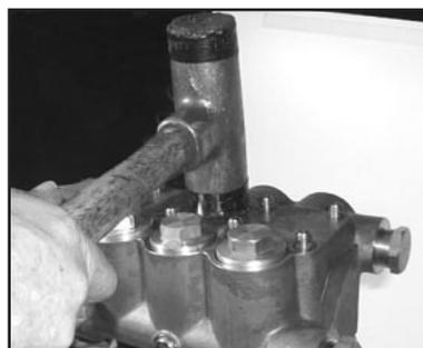
10. Place entire manifold/seal sleeve assembly over the studs and push firmly until seated against the crank-case.
