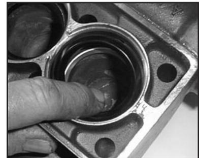
9. Place support ring (41) and v-sleeves (40) into valve casing.
