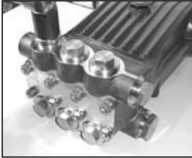
1. With a 30mm wrench, remove the six (6) plugs (48) from the valve casing (43). Inspect the O-rings (48A) and replace if necessary. Remove the complete valve assembly (46A) by threading a 12mm bolt into the spring retainer and pulling straight out.
