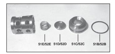
Check surfaces of valve plates (51D and 52D), valve seats (51C or 52C) and o-rings (51B and 52B). Replace worn parts.
